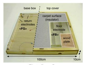
**Fig. 5.** Carpet Box (left) Return electrode strips / (right) Floor top electrode (covered)
