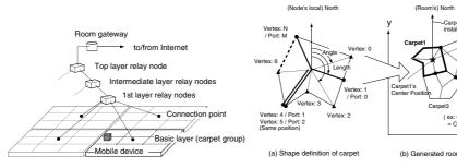
Fig. 8. Structure of CarpetLAN Network
