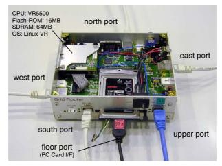
Fig. 12. CarpetLAN Node Linux-based six-port node unit
