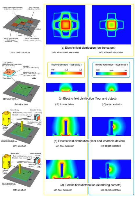
Fig. 4. Electric Field Simulations of CarpetLAN
