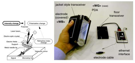
**Fig. 2.** EO Sensor **Fig. 3.** Transceivers Laser-beam is used for sensing. (L) Handy trx (in PDA's jacket) / (R) Floor trx
