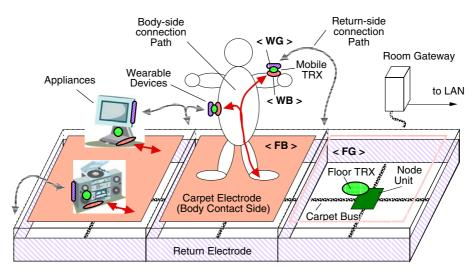
**Fig. 1.** System architecture. Each carpet-unit works as a network cell.
