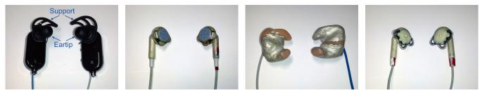
Figure 1. Prototypes tested. Starting from the left, "Rubber", "Disc", "Mold" and "Spring". Each pair of earphones has at least 3 independent electrodes.
