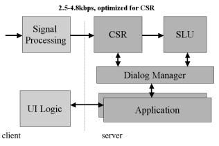
Figure 2MiPad'sclient -serverarchitecture.Theclientis basedonaWindowsCE iPaq,andtheserverisbasedon aWindows2000 machine.Thec lient-server communicationiscurrentlybasedonthewirelessLAN.
