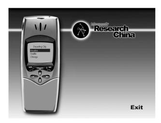
*Figure* 1: A multimodal smart phone prototype created using the SAPI 5.0 SDK.
