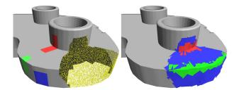
Fig. 23. Reconstructing part of a CAD model from sparse samples by copying matching parts from the model itself.
