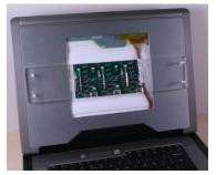
Figure 1: ThinSight enables multi-touch sensing using novel hardware embedded behind an LCD. Left, multi-touch input on a regular laptop LCD. Top row, the sensor data after interpolation, normalization, binarization, and component analysis. Bottom middle, front of three sensor boards tiled. Bottom right, sensors in position behind the display.
