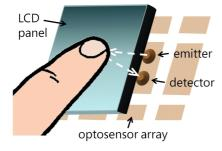
Figure 2: The basic construction of ThinSight. An array of retro-reflective optosensors is placed behind the LCD panel. Each of these contains two elements: an emitter which shines IR light through the panel; and a detector which picks up any light reflected by objects such as fingertips in front of the screen.
