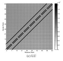
Figure 1: Communication traffic in CG, MG and LU (CLASS=C, NPROCS=64). The cell at (i, j) represents the communication volume (in bytes) between process i and j using shades of gray. With replay groups in sets of 8 sequentially numbered processes, intra-group messages account for about 77%, 55% and 50% of application communication traffic, respectively.
