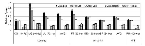
Figure 6: Record and replay speeds relative to base execution time (beside the application name on the *x*-axes). *Data Log, SRR log* and *Order Log* mean the record phases for data-replay, SRR and order-replay respectively. *AVG*: geometric mean for applications of the current communication pattern.
