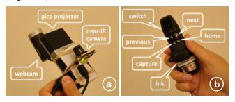
Figure 2: (a) AnatOnMe projection and capture device; (b) AnatOnMe input device: a modified presenter.
