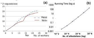
Figure 5: (a) Pairs of requests executed per second at the cloud as depending on the number of workers. (b) Auditing performance for one owner node.
