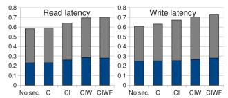
Figure 3: End-to-end and effective read and write latency. Each bar indicates the end-to-end latency incurred, with the darker section showing the effective latency.
