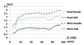
Figure 6: The duration of a membership update as depending on the number of members with access to a block family.
