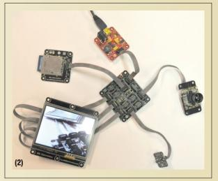
Figure A. Creating a digital camera using .NET Gadgeteer: (1) the graphical configuration tool and (2) the corresponding hardware.
