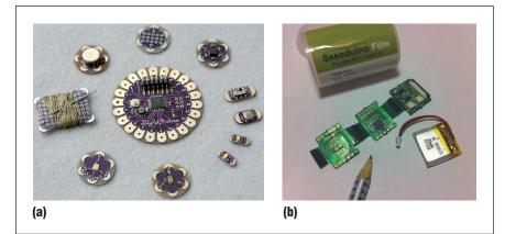
Figure 2. Arduino has revolutionized electronics development, and a very active community has evolved the hardware platform from the original standard printed circuit board (PCB) form-factor to include (a) wearable devices, such as Lilypad (photo courtesy of Leah Buechley) and (b) very small, flexible devices, such as Seeeduino film.
