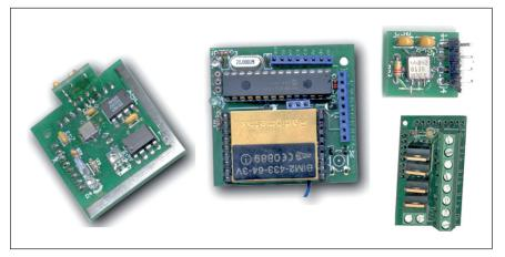
Figure 1. Smart-Its—an early prototyping platform developed in 2001.
