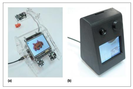
Figure 3. Two devices built with Microsoft's .NET Gadgeteer platform. Both contain similar components, but the different physical arrangements greatly influence the affordances of each device. (a) The stop-motion animation unit, which has a camera mounted on an adjustable arm, and (b) the telepresence device, which has a fixed camera pointing at the user. Rapid prototyping technologies such as laser-cutting and 3D printing are of great help here.
