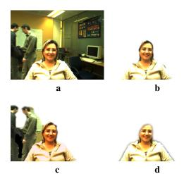
Figure 8. Segmentation results on the "IU" test sequence. (a) Original, (b) stereo-based segmentation from [8], (c) monocular segmentation from [5], where background motion pops into foreground, (d) monocular segmentation from the proposed algorithm.
