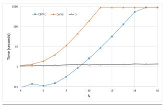
**Figure 3.** Comparison of BMC tools against DAG Inlining (DI) on the program of Fig. 2, under a timeout of 900 seconds.
