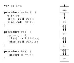
Figure 2. A program parameterized by the value of N and an illustration of DAG inlinig for N=3
