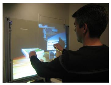
Figure 1. Interacting with DepthTouch: user's left hand is touching an object of interest, while his right hand is adjusting the orientation and depth of that object by moving in mid-air above the surface.
