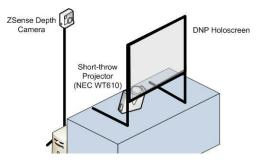
Figure 2. DepthTouch system components.
