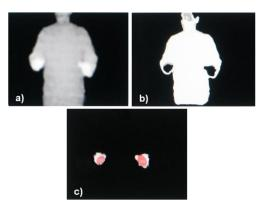
Figure 3. Segmenting the user's body using depth values: a) the depth image of the user standing in front of the screen, b) the torso image shows segmented body without the outstretched hands, and c) the hands image showing segmented arms and hands that can now be easily tracked.
