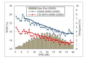
Figure 3: Performance comparison of the CD-GMM-HMM and CD-DNN-HMM at different SNR levels for the SMD task.
