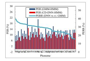
Figure 1: Phone error rate (PER) of the CD-GMM-HMM and CD-DNN-HMM rendered by ordering the phonemes by the decreasing order of phone error rate reduction (PERR).
