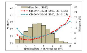
Figure 7: Performance comparison of the CD-GMM-HMM and the CD-DNN-HMM at different speaking rate for the SMD task.
