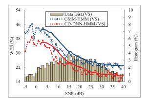
Figure 2: Performance comparison of CD-GMM-HMM and CD-DNN-HMM at different SNR levels for the VS task.
