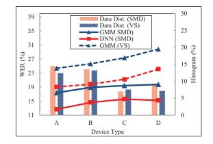
Figure 4: Performance comparison of CD-GMM-HMM and CD-DNN-HMM models on four different devices.
