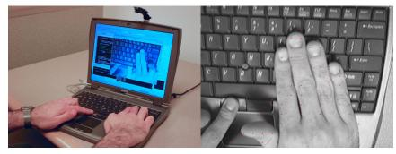
Figure 1 Left: FlowMouse prototype with screen-mounted camera facing down on keyboard and user's hands, and touch sensitive strip on left mouse button. Right: Example image capture from camera.
