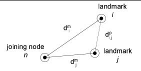
Figure 9. Triangle inequality with measured and predicted distances.
