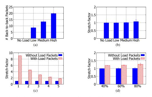
Figure 4: (a) Number of back-to-backs, and (b) *stretch-factor* with varying wireless congestion levels. *stretch-factor* for WAN link bottlenecks due to (c) varying link bandwidth (in Mbps) and (d) varying cross-traffic volumes.
