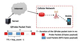
Figure 2: QProbe packet train with tiny probe packets and large load packets. TTL for load packets expires 1-hop before cellular network and get dropped en route.
