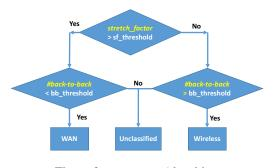
Figure 3: QProbe Algorithm
