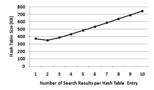
Figure 8: The memory footprint of the hash table as a function of the number of search results per hash table entry. For all data points we used exactly the same < query, link, score > triplets that correspond to 60% of the cumulative query-link volume (Figure 4).
