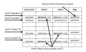
Figure 7: The hash table data structure used to link queries to search results.
