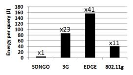
Figure 14: Average energy per query when SONGO and different radio links are used to serve search queries.
