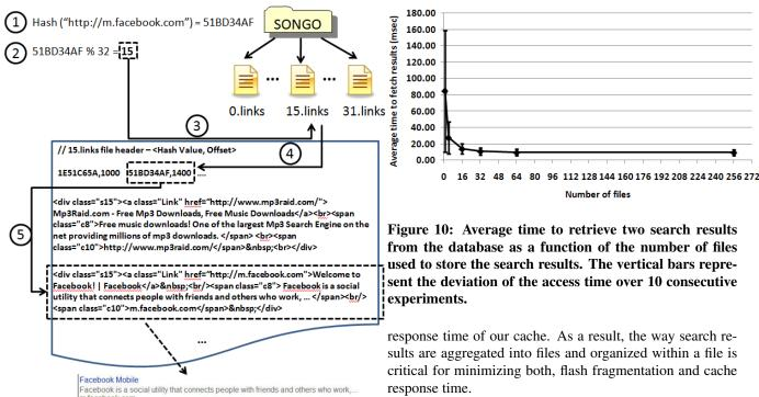
Figure 9: Search result database structure and illustration of the process of retrieving a search result when N = 32 files are used.
