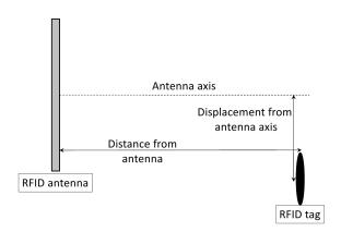
Figure 3: Measurement setup
