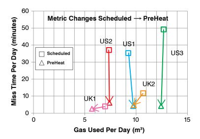
Figure 1. Compared to setting a daily schedule with a programmable thermostat, PreHeat saved 8% and 18% on gas usage in the two U.K. homes. In the three U.S. homes, PreHeat did not save as much, but rather used the gas more effectively: It was less likely the house would be below the set temperature while occupied (Miss Time on the y axis).
