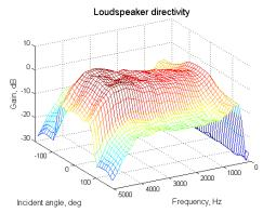
Figure 2. Loudspeaker magnitude response.
