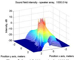
**Figure 5.** Sound field intensity for 1000 Hz.
