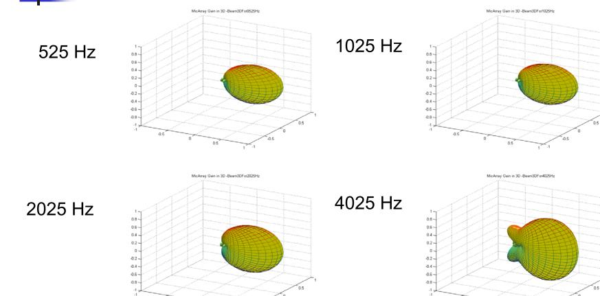
The beam shape in 3D proves frequency independent beamforming
