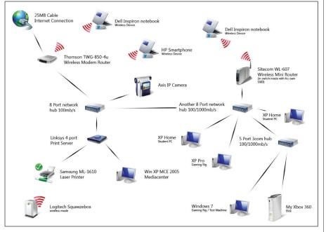
Figure 1. Schematic of real home network.
