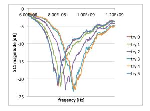
**Figure 5.** The resonant frequency of the printed antenna was initially 807 MHz. Following successive erasure of ink to reduce the length of the dipole (tries 1-4), it changed to the target frequency of 918 MHz. Then ink was reapplied using a pen (try 5) and resonance returned to the original frequency.
