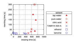
**Figure 3.** Erasing and rewriting time when using a melamine sponge bathed in a range of solvents.
