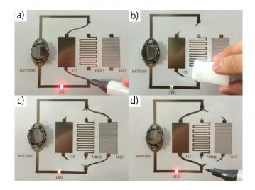
**Figure 1.** Circuit Eraser can be used to remove conductive patterns which are hand drawn or inkjet printed. It is possible to re-apply conductive ink in the same region if necessary.
