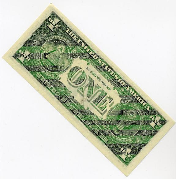
Fig. 4. Selective mis-rendering of obverse of US currency. Observe that the bands are visible even if printed at an angle.
