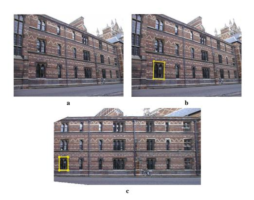
**Figure 9:** Rectifying planar structures in photographs. (a) A photograph of the Keble College in Oxford, UK. (b) Original photo with four selected points superimposed. The selected points are used to compute the homography between the scene plane and the image plane. (c) The automatically rectified image. The wall appears to be viewed from a front-on position. See text for details.
