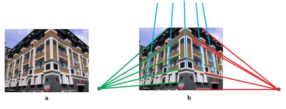
**Figure 1:** In a photograph parallel scene lines are imaged as converging lines. (a) A photograph of a building in Cambridge, UK. (b) Three sets of parallel lines (in green, blue and red) are shown. In the image plane all the lines in each set converge into a single point, namely the vanishing point. The vanishing point associated with the set of lines shown in blue falls well outside the image.
