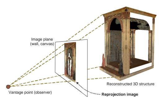
**Figure 25:** The reprojection image is defined as the image created by projecting the computed three-dimensional reconstruction onto the plane of the painting.
