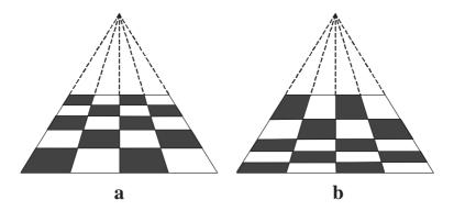
**Figure 4:** A drawing of a tiled floor. (a) The tiles are perceived to be the same size. (b) The tiles are not perceived to be equal size. In this case the rate of diminution of the images of the tiles is not consistent with the assumption that all the tiles have the same area. Despite the fact that in both cases the "orthogonals" correctly converge into a single vanishing point, our brain does not perceive the second as an image of a slanted floor.
