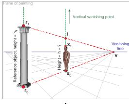
**Figure 6:** Measuring heights in paintings. (a) We wish to compute the height of the human figure relative to the height of the column. The vanishing line of the image is supposed to have been computed (shown in blue). (b) The ratio between the height of the man and that of the column is given by  $\frac{h}{h_T} = d(\mathbf{x}_t, \mathbf{x}_b)/d(\mathbf{i}, \mathbf{x}_b)$ . See text for details.
