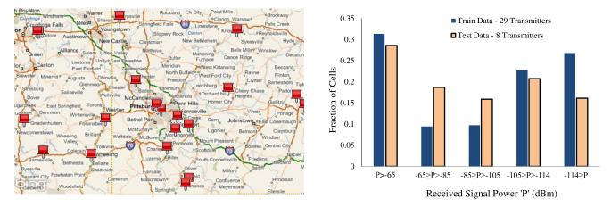
**Figure 6.** (a) Transmitters in parts of Southwest Pennsylvania / East Ohio. (b) Distribution of received signal for the training and testing data in Southwest Pennsylvania.
