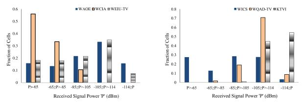
Figure 3. Distribution of received signal powers from six DTV transmitters in Illinois.
