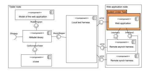
Fig. 3. A SysML component diagram of the setup of model-based testing of a web application.
