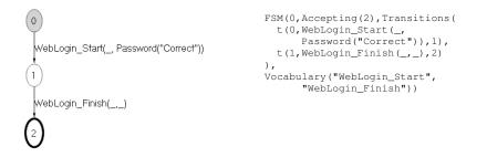
Fig. 2. A login scenario restricting the behaviour to only trying correct passwords.
