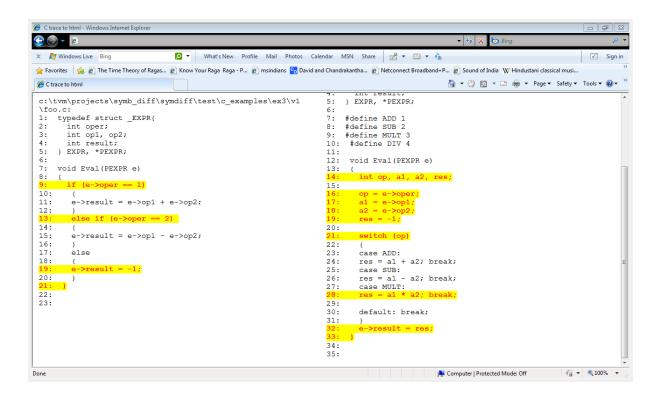
Figure 1: Output of the symbolic diff tool [7]. The highlighted statements indicate a path in the two versions of a program, where the procedure has different side effects.
