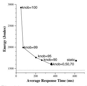
This graph shows average response time and total energy used by the e-mail reader for seven different STPM knob values. Knob values from 0 to 70 yield equivalent results. For reference, the static disk cache strategy is also shown. The dotted line on the bottom graph is a lower bound on the minimum energy needed to execute the trace.
