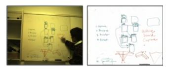
**Figure 5.** Live whiteboard capture. The image on the left is one of the raw image sequence captured by the whiteboard camera; the image on the right is the processed and enhanced image.
