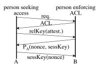
Figure 5: Checking the attestation of a person seeking access. The attestation is encrypted with the attestation's relationship key before sending it. The nonce exchange checks that the person seeking access has the private key corresponding to the public key of the attestation's recipient.
