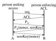
Figure 4: Checking the identity of a person seeking access. The ACL enforcer checks that the person's public key appears in the ACL's explicit list of users with access to the object. The nonce exchange checks that the person has the private key corresponding to the public key sent earlier.
