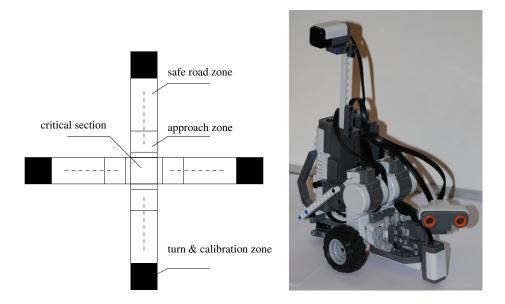
Fig. 1. The intersection that constitutes the environment for the mobile robots (*left*) and an implementation of a mobile robot for the intersection example (*right*).
