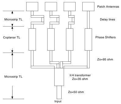
Fig.1: Block diagram of a 4-element steerable array antenna.
