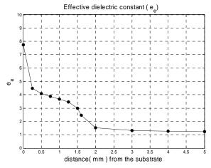
Fig. 3: Effective dielectric constant as a factor of distance from the substrate.
