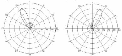
Fig. 5: Radiation patterns of a 4-element array antenna shown in Fig. 1. The initial phase is shifted to create  $-90^{\circ}$  phase difference at d=0 mm (left figure). At d=5 mm, the phase difference becomes  $+90^{\circ}$  (right figure).
