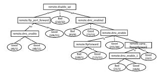
Figure 4: NetPrints configuration tree for the FTP client.
