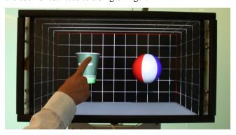
Figure 8. 3D contour tracing application where the user feels the shape of the 3D object by tracing their finger along its surface. Note: stereo rendering is disabled for clarity.
