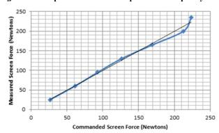
Figure 6. Plot of measured force vs. commanded force.
