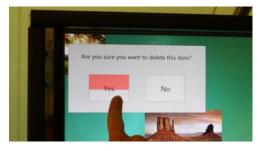
Figure 10. An example of touchscreen interactions augmented with kinematic haptics. Z-buttons (e.g., Yes confirming deletion) require higher force and larger displacement of the screen than others to eliminate accidental activation. The button rendering serves as a progress bar, visually reinforcing the amount of movement necessary to complete the action.
