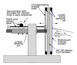
Figure 2. Simple diagram outlining major components of the TouchMover device.
