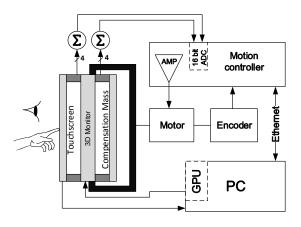
Figure 4. TouchMover system schematic.
