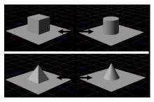
Figure 15. Examples of shapes that are difficult to disambiguate from only 1D haptic feedback in our system. Not being able to haptically render vertical edges (cube) or mostly vertical edges (pyramid) makes such objects confusable with similar shapes that don't have vertical edges (cylinder and cone respectively).
