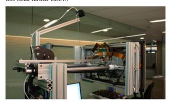
Figure 3. Image of the back side of our device showing the rack and pinion gear and the completely supported 3D touchscreen up front (consult Figure 2 for explanation of the components).
