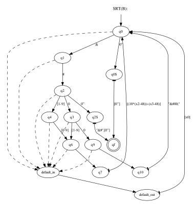
Fig. 2. Sample SRT with rollback-transitions.
