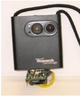
(a) SenseCam with added compass sensor
