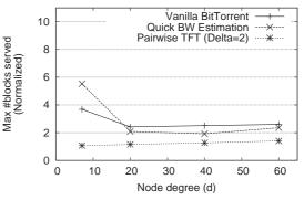
Figure 4: Maximum number of blocks (normalized by file size) served by any node with the bandwidth-matching tracker policy in use for (a) vanilla BitTorrent (but for the new bandwidth-matching tracker policy), (b) BitTorrent with QBE, and (c) with the pairwise block-level TFT policy. Compare with Figure 2.
