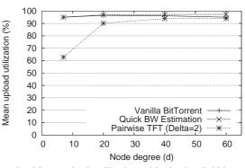
Figure 3: Mean upload utilization with the bandwidth-matching tracker policy in use for (a) vanilla BitTorrent (but for the new bandwidth-matching tracker policy), (b) BitTorrent with QBE, and (c) with the pairwise block-level TFT policy. Compare with Figure 1.
