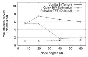
Figure 2: Maximum number of blocks (normalized by file size) served by any node during an experiment for (a) vanilla BitTorrent. (b) Bit-Torrent with QBE, and (c) with the pairwise block-level TFT policy.
