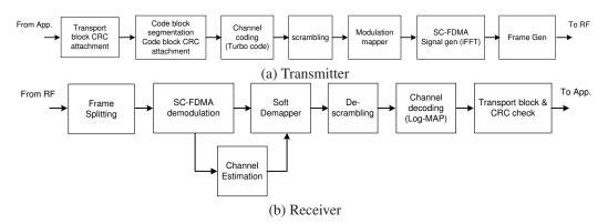
Figure 2: Illustration of LTE PUSCH transceiver.
