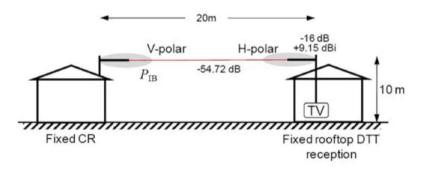
Figure 20: Reference geometry 2 for a fixed 10m WSD device to a 10 m DTT antenna
