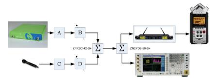
Figure 24: Radio Microphone Bench Test Configuration
