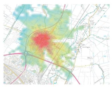
Figure 14: UKPM Coverage Prediction for CH 61 BS Coverage
