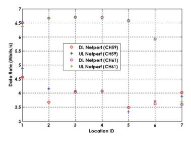
Figure 15: Throughput comparison between Channel 59 and Channel 61
