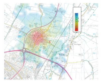
Figure 13: UKPM Coverage Prediction for CH 59 BS Coverage
