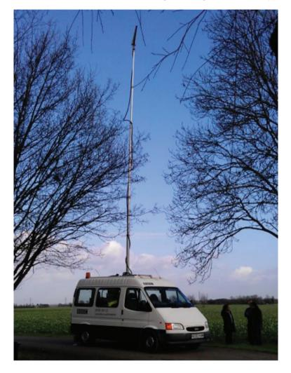
Figure 12: BBC R&D survey vehicle with elevated mast at 10 m Photo: Mark Waddell
