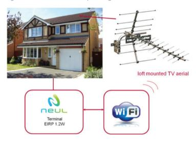
*Figure 17: The residential property in Orwell, where a White Space to Wi-Fi bridge was installed*
