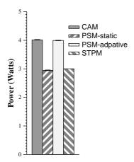
These graphs show how the choice of power management policy affects the power used to play streaming audio on an iPAQ using XMMS. Each bar shows the mean of three trials—the error bars show the value of the minimum and maximum trial
