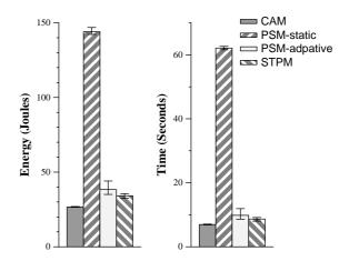
These graphs show how the choice of power management policy affects the time and energy needed to run remote X applications. The rightmost graph shows the time to start the Gnumeric application running on the server with the display on the iPAQ client, load a spreadsheet, and close the application—the leftmost graph shows the total energy expended. Each bar shows the mean of three trials—the error bars show the value of the minimum and maximum trial.
