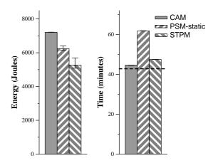
These graphs show the time and energy needed to execute NFS operations using a Orinoco Silver 802.11b card. These results can be compared to those in figure 10 for the Cisco Aironet 350 card. It is not possible to disable the Orinoco card, nor does it support an adaptive PSM. Each bar shows the mean of three trials—the error bars show the value of the minimum and maximum trial.
