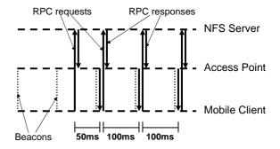
Figure 2: RPC delays due to power management
