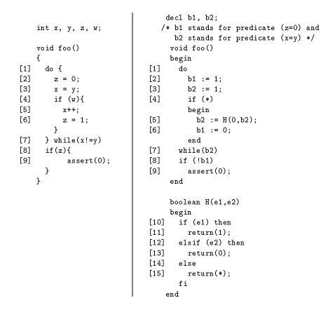
Fig. 1. An example C program, and the Boolean program produced by c2bp using predicates (z=0) and (x=y)
