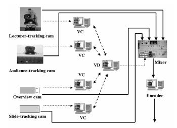
Figure 1. System block diagram. Dashed lines indicate status and command signals. Solid lines indicate video data. VC stands for virtual cinematographers and VD stands virtual director. One thing worth pointing out is that even though we represent various VCs and VD with different computers, they can actually reside in a single computer running multiple threads.
