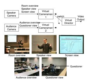
Fig. 7. The video capturing process.
