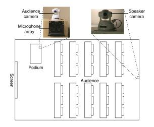
Fig. 4. A typical configuration of the  $iCam\mathcal{2}$  system.
