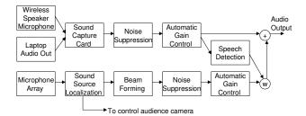
Fig. 5. The audio capturing process.
