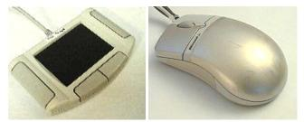
Fig. 1 Input devices for our desktop two-handed interaction techniques: a touchpad for the nonpreferred hand and the TouchMouse, a modified Microsoft IntelliMouse that can sense when the user is touching it.
