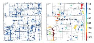
Figure 11. Candidate parking places (left) and clustered parking places (right) in the area of Beijing West Railway Station. The color indicates the number of parking candidates detected for each cluster.
