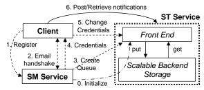
Fig. 4. Interaction between a client, SM, and ST. The various operations are numbered in the order in which they are invoked. The dashed-dotted line operation (#0) is invoked at system initialization time. The dashed line operations (#1-#5) are invoked at the time of client registration. The solid line operation (#6) is invoked during normal operation, i.e., posting and retrieval of notifications.
