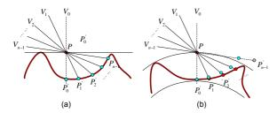
Figure 3: View-dependent displacement variation for curved surfaces.
