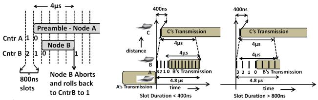
Figure 4: Making slot duration independent of carrier sensing time
