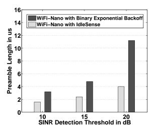
Figure 13: Preamble length for different detection thresholds
