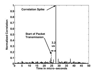
Figure 8: Carrier Sensing Using Pseudo-Random Preamble
