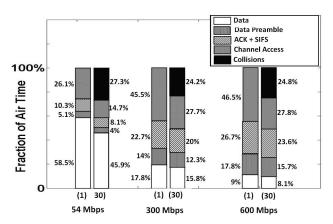
Figure 2: Overheads at different data rates
